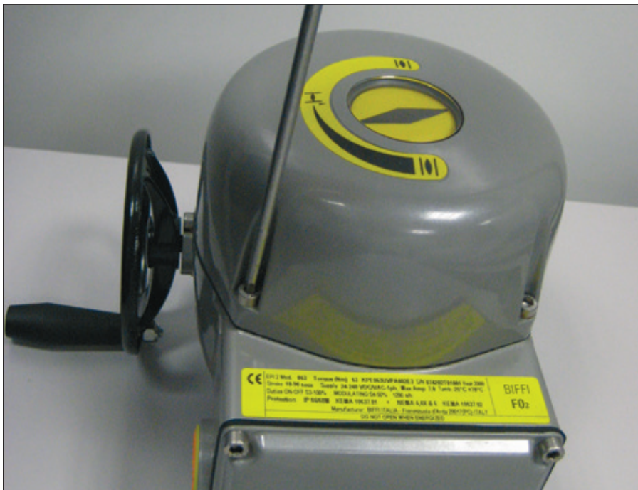
FIGURE 14 - Removal of the control unit cover.
