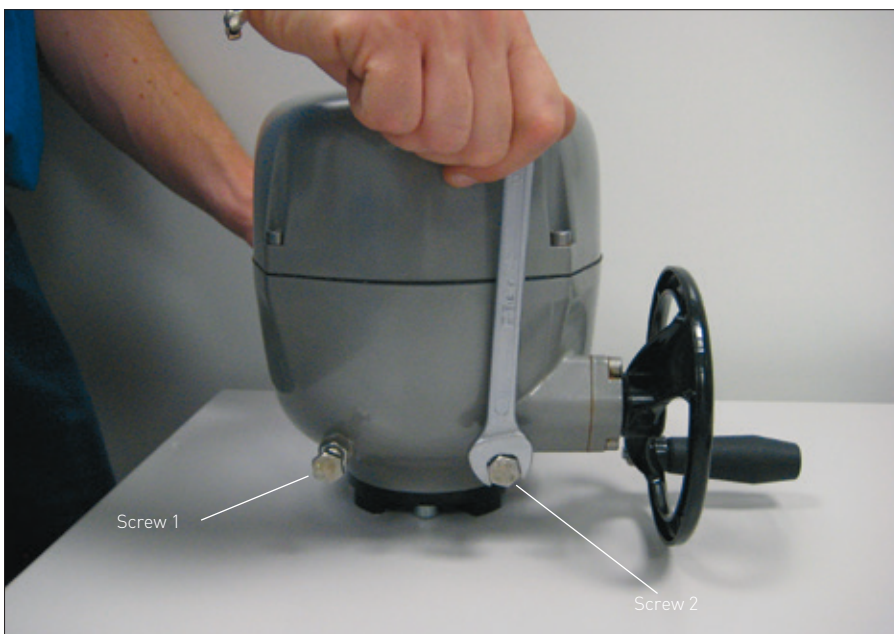
FIGURE 7 - Setting of the mechanical stop.
